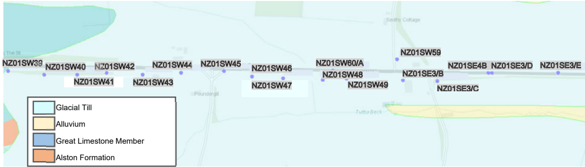
Figure 2: Pounder Gill to Cross Lanes Borehole Locations and Superficial Geology [11].
